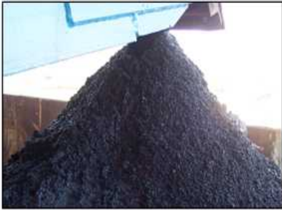
Figure 9. Gasifier Slag to Roll-Off Container.
