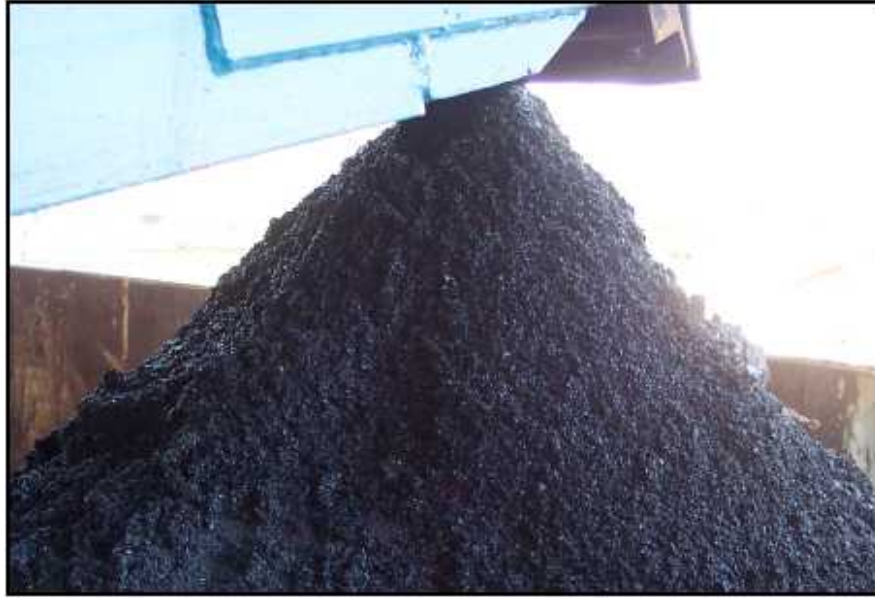
Figure 8. 1 st Stage Combustor Slag to Roll-Off Container.
