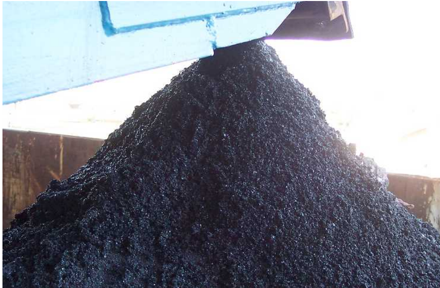
Figure 7. 1 st Stage Combustor Slag to Roll-Off Container.
