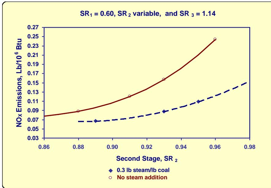
Figure 6. Three Stage Kinetic Modeling NO<sub>x</sub> emissions prediction.
