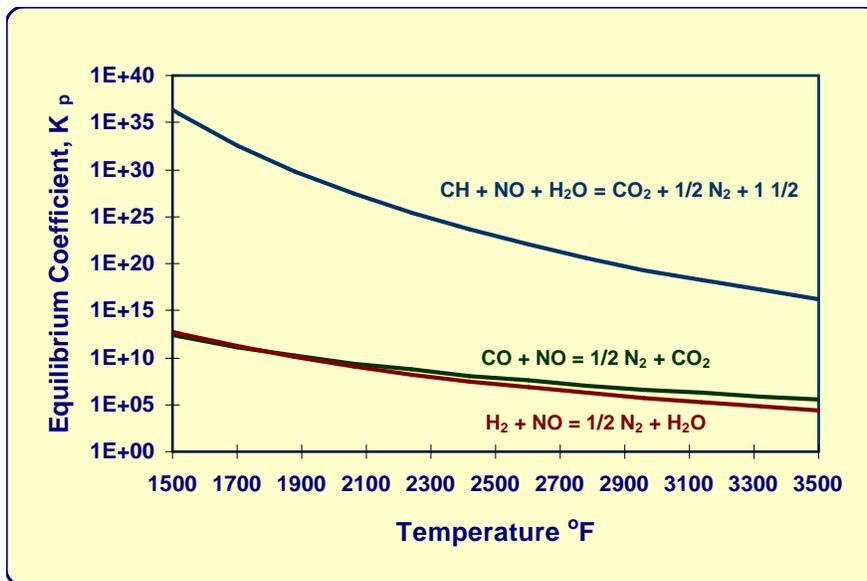
Figure 4. 2<sup>nd</sup> Stage NO reducing reactions.
