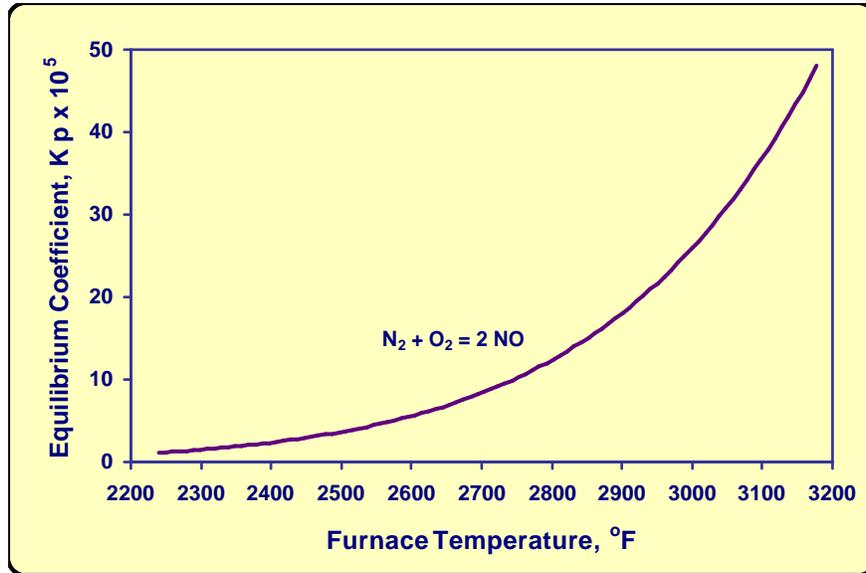
Figure 5. 3<sup>rd</sup> Stage NO formation thermochemical equilibrium.
