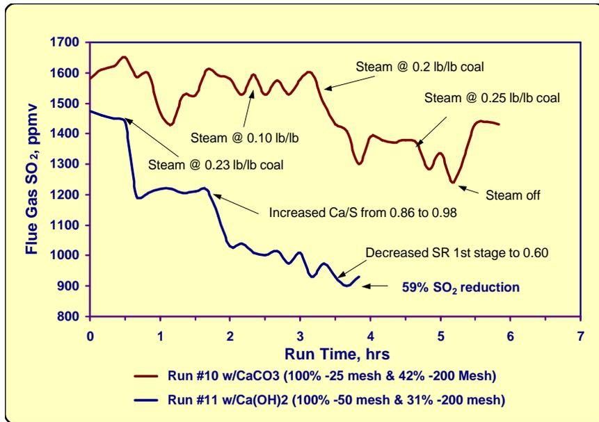
Figure 1. Flue gas SO<sub>2</sub> concentration versus run time.
