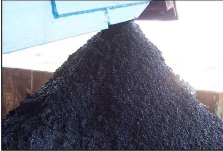
Figure 8. 1<sup>st</sup> Stage Combustor Slag to Roll-Off Container.
