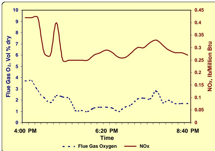
Figure 2. NO<sub>x</sub> emissions reduction as a function of 2<sup>nd</sup> Stage flue gas oxygen.
