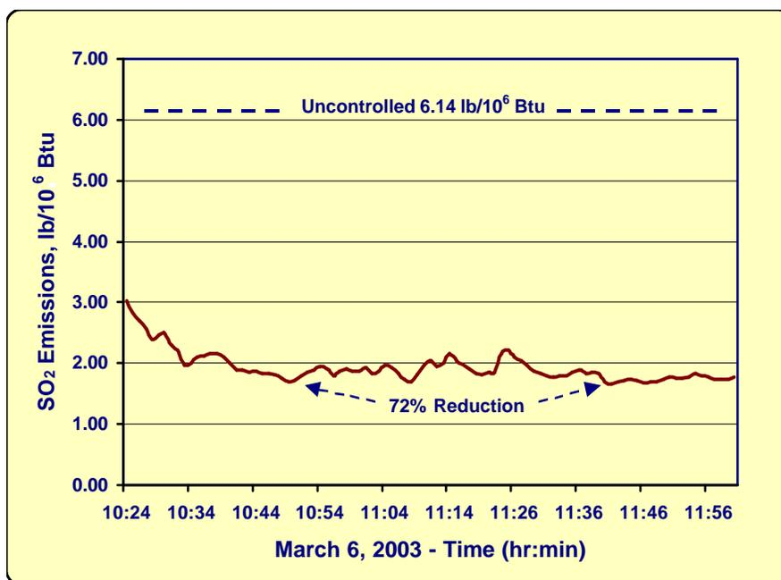
Figure 10. SO<sub>2</sub> reduction at Lincoln.
