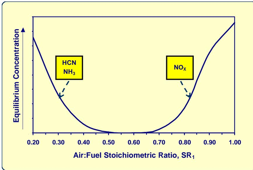
Figure 3. 1<sup>st</sup> Stage HCN, NH<sub>3</sub> and NO<sub>x</sub> relative equilibrium concentrations.
