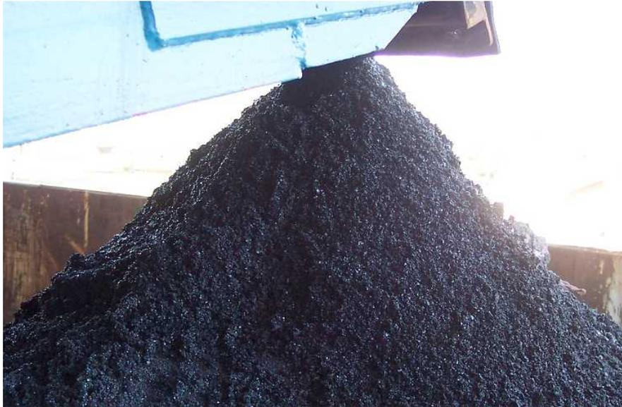
Figure 7. 1<sup>st</sup> Stage Combustor Slag to Roll-Off Container.
