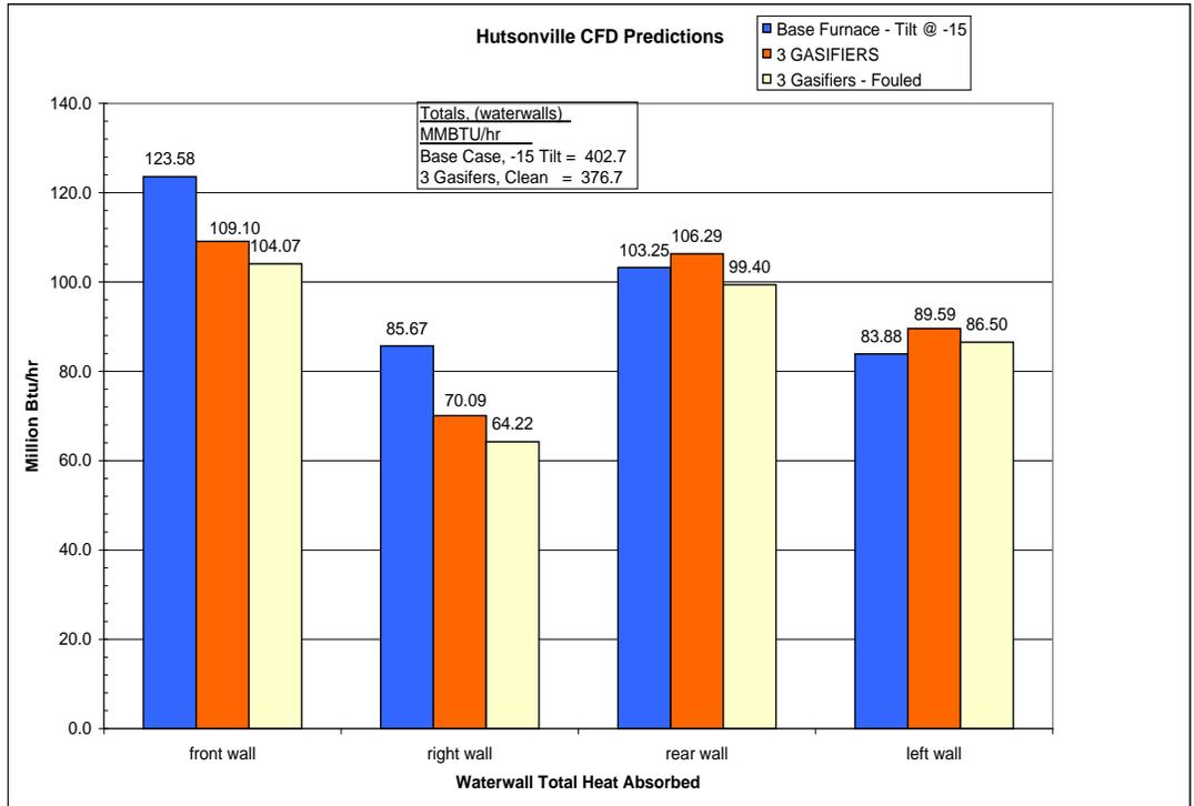
**Figure 3. Heat absorption comparison.**
