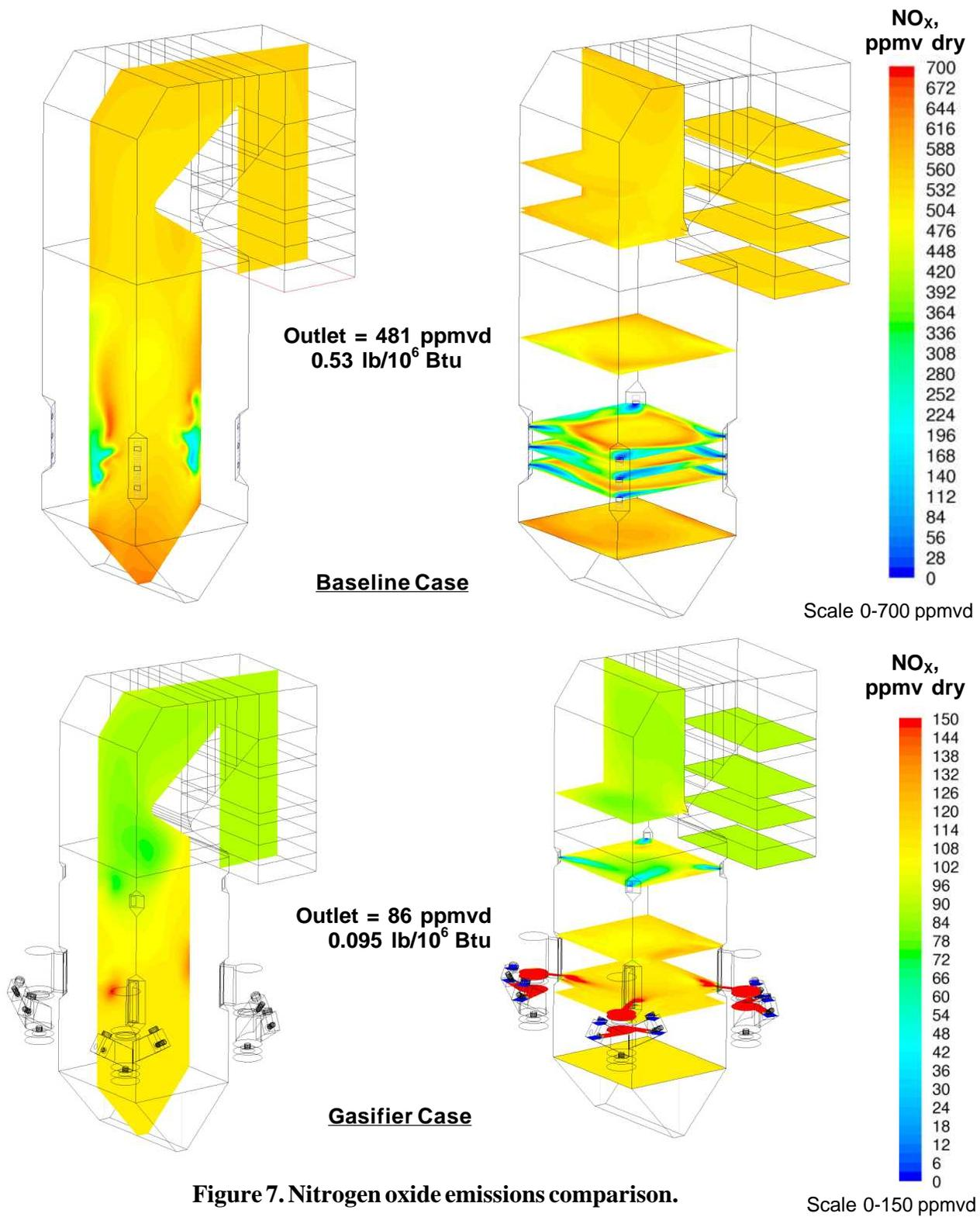
**Figure 7. Nitrogen oxide emissions comparison.**
