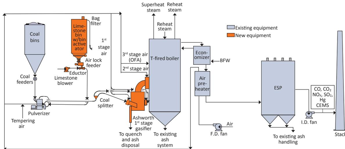
FIGURE 1. Ashworth Gasifier-Combustor retrofit schematic
